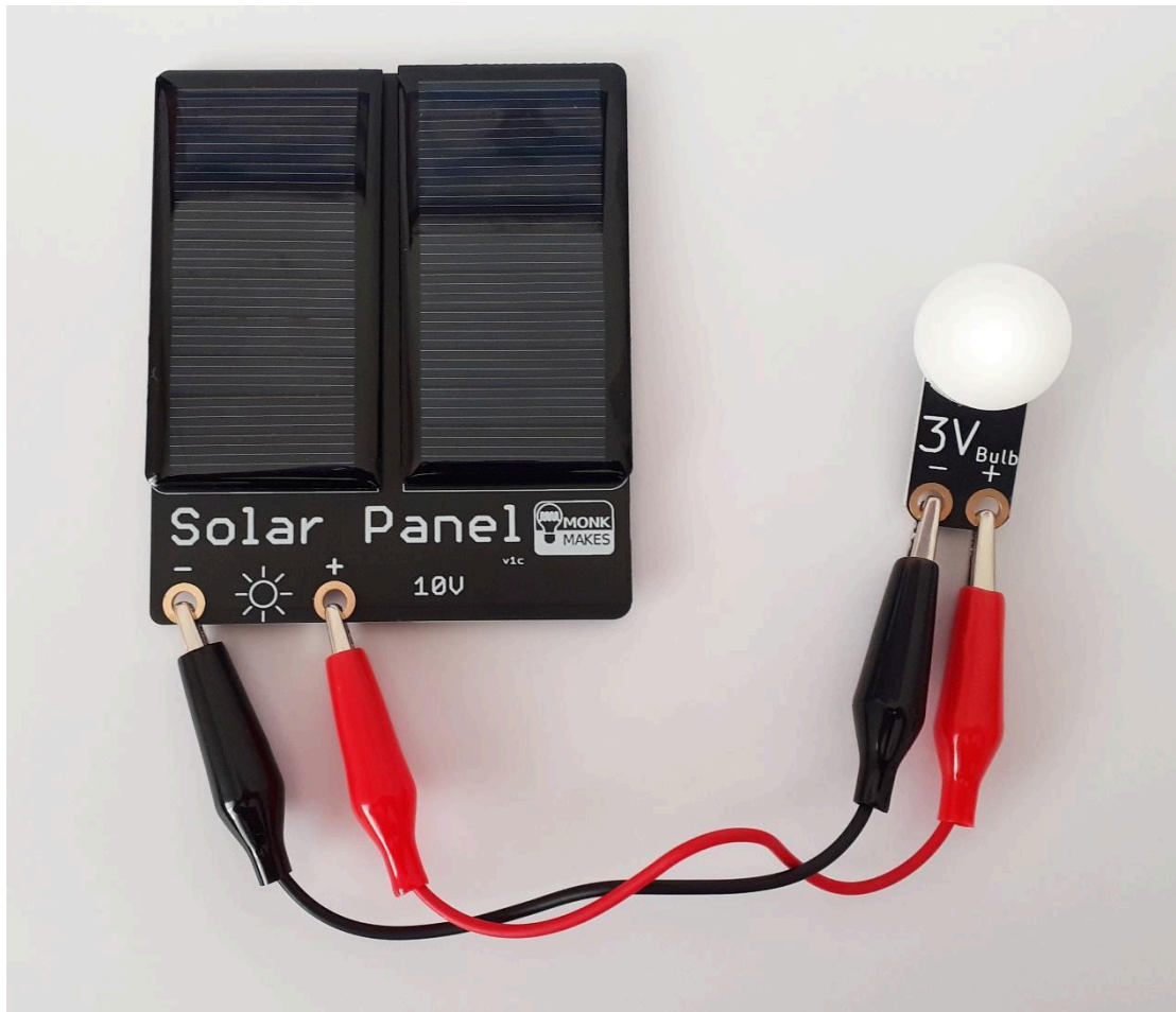
Figure 1: Connecting the LED light to the Solar Panel by using two alligator clips. Connect the + and – terminals of the Solar Panel to the + and – terminals of the LED light.
