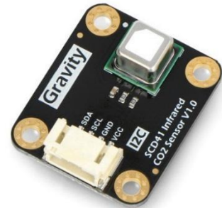
Figure SEQ Figure \* ARABIC 3. SEN0536 module for CO2, T and H (source: manufacturer)
